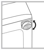
2. If the floor is not perfectly level, compensate for any unevenness by tightening or loosening the adjustable front feet (see figure); the angle of inclination, measured according to the worktop, must not exceed 2°.
